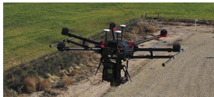
Figure 8.6: Drone leak detection
