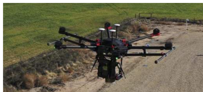
Figure 8.6: Drone leak detection
