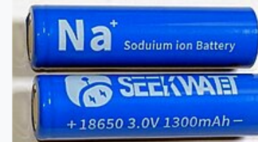
A sodium-ion cell (size 18650)
